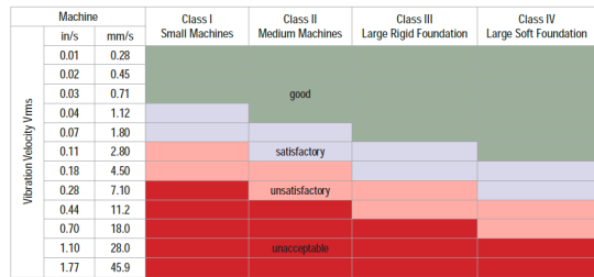
Figure 1. Vibration Severity per ISO 10816
