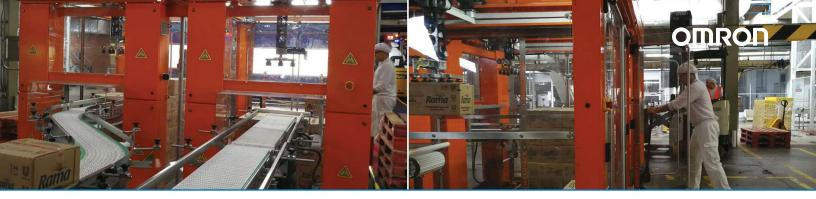
To maximize pallet space while ensuring stability of loaded pallet is critical for both reducing cycle time and maximizing worker safety. The synchronized movement of the cartesian system's four axes with all motion servos allows for the best route selection with a smooth trajectory, no matter the package coming down the variable speed conveyor.
